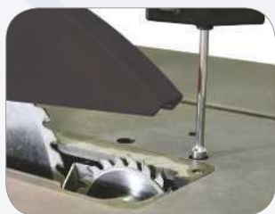
Easy access to pre-scoring adjustment
